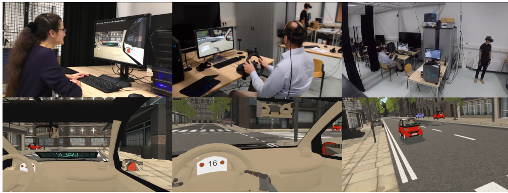
Figure 1: Multi-agent crossing scenario in coupled simulator [2]: AV passenger, MDV driver, and pedestrian (top); views of the three agents (bottom).
